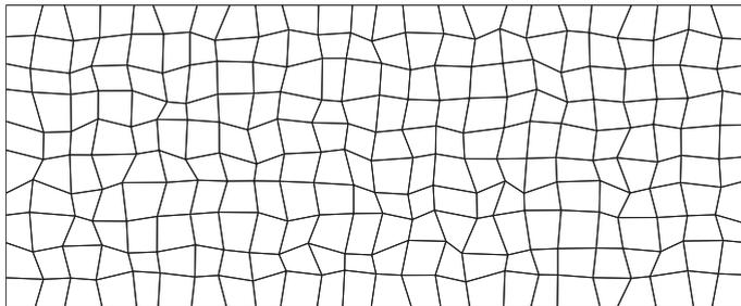
**Fig. 5.** Coarsest regular mesh used in the SWE with a manufactured solution; (a) triangular mesh, (b) rectangular mesh, and (c) Skew-rectangular (quadrilateral) mesh.
