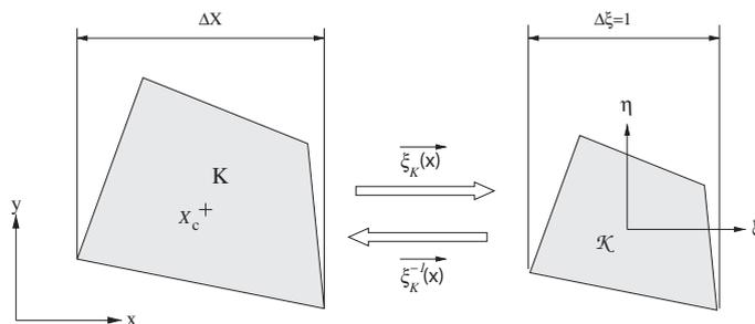
Fig. 2. Schematic diagram of the coordinate transformation.
