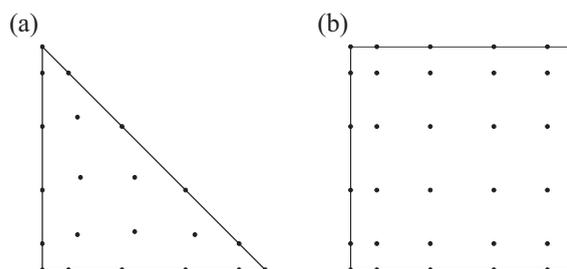
Fig. 4. Distribution of interpolation points on the master elements with  $p = 5$ : (a) triangular element, and (b) rectangular element.
