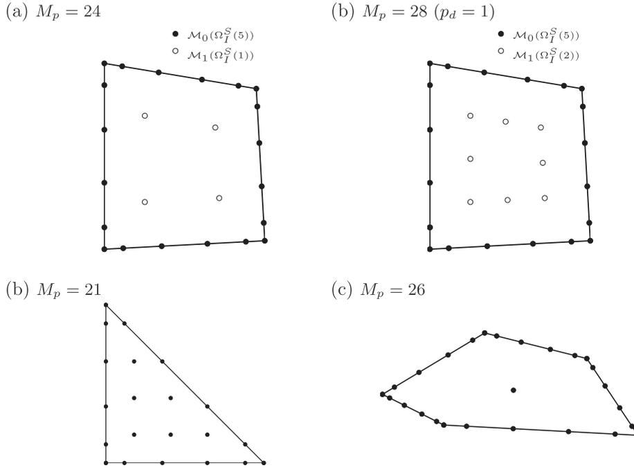
**Fig. 3.** Nodal distribution for  $p = 5$  ( $N_p = 21$ ): (a) quadrilateral element with  $p_d = 0$  (b) quadrilateral element with  $p_d = 1$  (c) triangular element with  $p_d = 0$ , and (d) pentagonal element  $p_d = 0$ .
