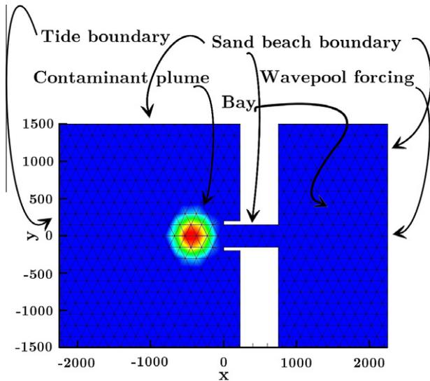
**Fig. 2.** Initial conditions, boundary conditions and course mesh of the contaminant plume declination model, where the bay is on the right with a wavepool forcing.
